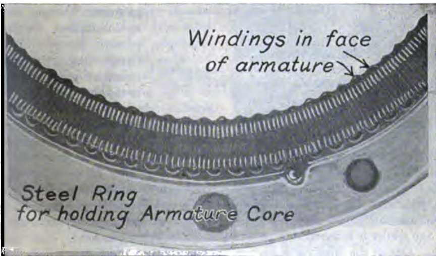
FIG. 15A.—A view of a section of one armature of the machine in Fig. 15.
